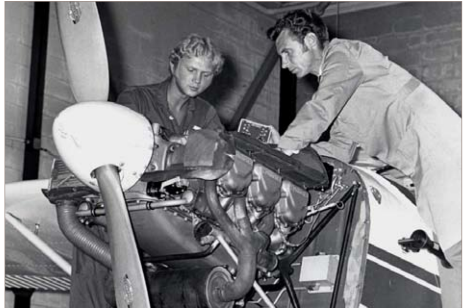
Student Dave Upton gets a lesson in how to time magnetos on a Cessna 180 from instructor Bill Foyle (right) in this photo from 1972.
