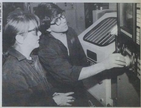
School of Trades students Irene Smith of Sechelt and Brad Johnson of Gold River check out the latest computerized lathe equipment in the Computer Numerical Control Lab at BCIT. Both are students in the Industrial Maintenance Mechanics Program. The Okuma LB15 lathe was recently donated to BCIT by Thomas Skinner and Son Ltd. It is valued at \$160,185.
