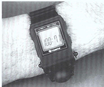
Blood-pressure device, developed by the Technology Centre, is worn as a wrist watch.
