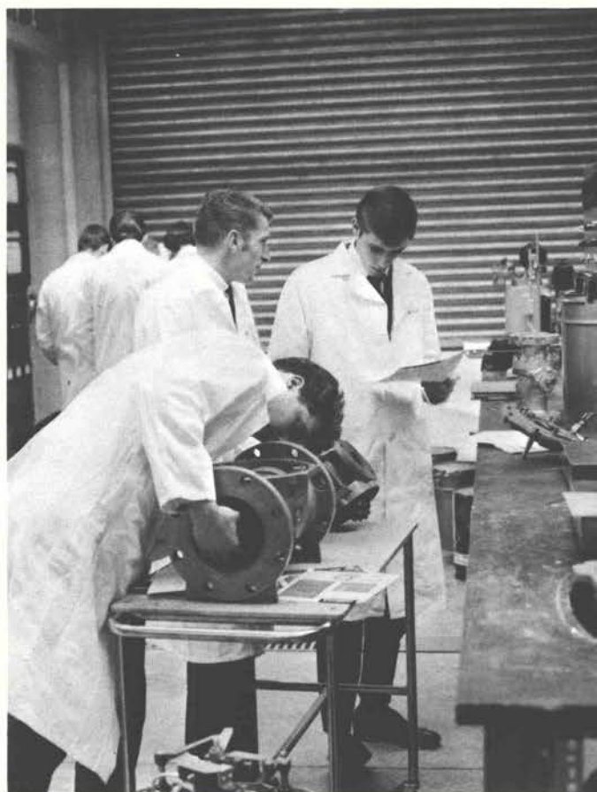
Inspecting a Turbine Flow Meter
