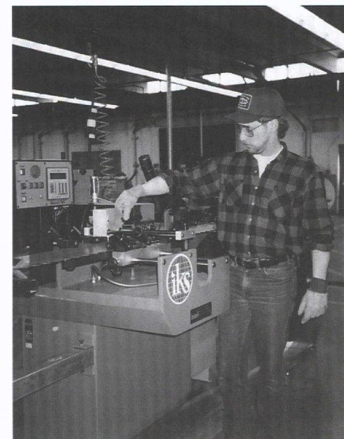
Saw Trades student training on the new automatic band saw leveler donated by International Knife and Saw.
