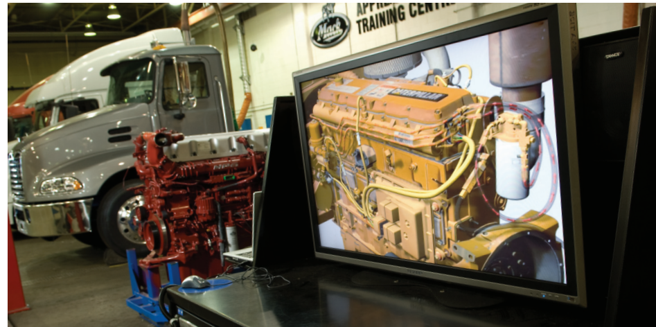
A 3-D MODEL IN THE NGRAIN VIEWER CAN BE ASSEMBLED, DISASSEMBLED, ROTATED, AND VIEWED IN CROSS-SECTION — ALL IN REAL TIME.
